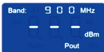
**LCD6:** Displays "-" if the output power is negative, **LCD7:** Gain or power indication.
