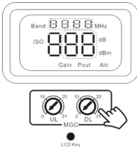
To start the operation mode press "LCD key" once.
