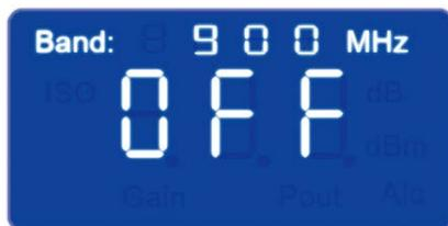
When LCD screen is in "OFF" state and the repeater shuts down, LCD screen will be flashing.
