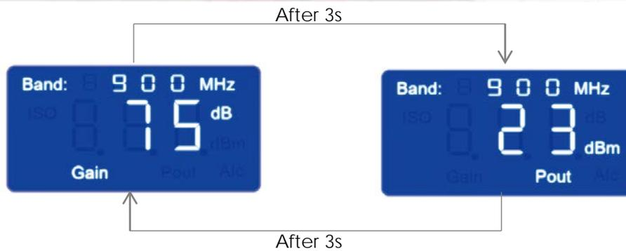
You can always press "LCD key" so that the LCD will stay in the output power mode, and in case it is dual band, you can press "LCD Key" to switch to another band's output power display.
